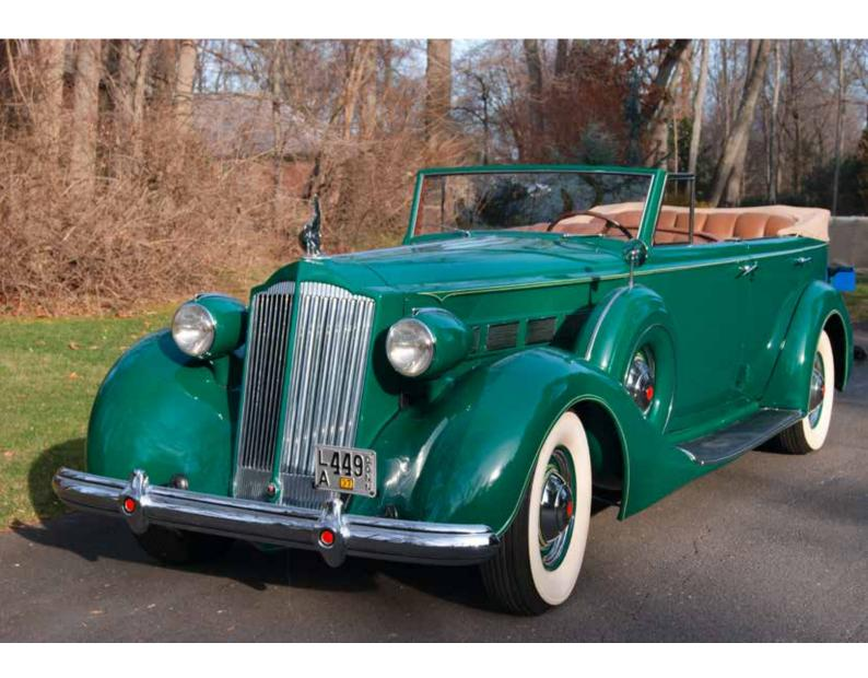
The eight-cylinder Packard was in its 15th series (there was no 13th) by the time this Model 1507 rolled off the Detroit company's production line in 1937. The big news for '37 was the introduction of the 5.2-liter engine on the larger Eight, which now incorporated independent front suspension and hydraulic brakes. All Packards had featured synchromesh transmission since 1933. Now, the radiator was tipped back with a 30 degree slant, giving it a more swept back look.
